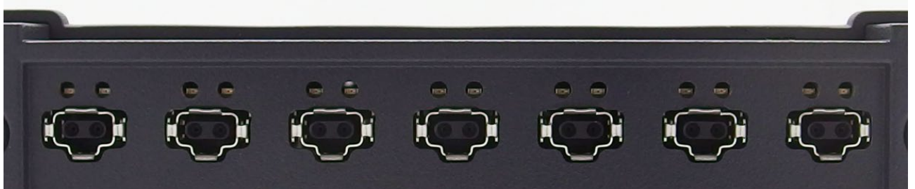
Figure 4: 1000BASE-T1 SPE connector side with LEDs
