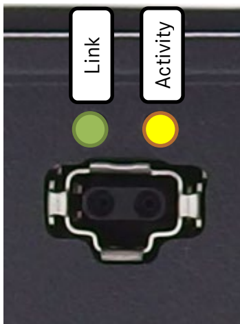
Figure 5: SPE-T1 Ethernet connectors Con 1 to Con 7 with yellow and green LED
