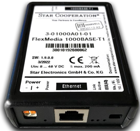
Figure 1: Side with Power and Ethernet (100BASE-TX/1000BASE-T)
