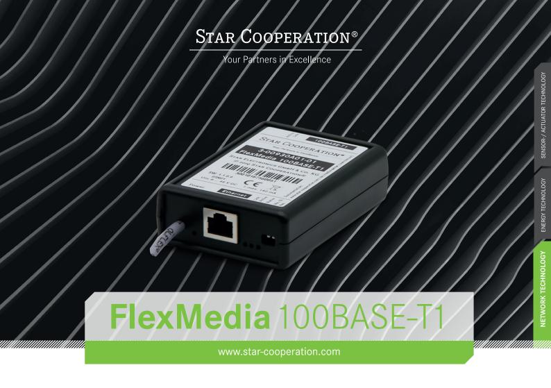
The FlexMedia 100BASE-T1 is a converter for 100BASE-T1 to 100BASE-TX and vice versa. With the FlexMedia 100BASE-T1, it is possible to connect an automotive Ethernet network to a standard PC for testing or diagnostic purposes. It supports up to 100 Mbit/s in full duplex mode on both sides.
