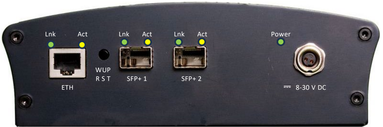
Figure 2: Power cover with 100BASE-TX, push button, 2x SFP+ and power connector
