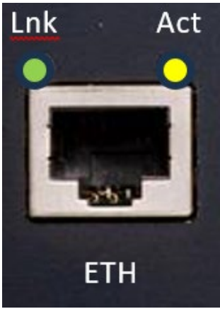
Figure 5: ETH Port, RJ45 connector with LEDs
