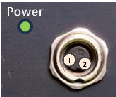
Figure 3: Power connector M9 2pol with LED
