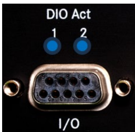
Figure 8: D-Sub DIO connector with two blue LEDs
