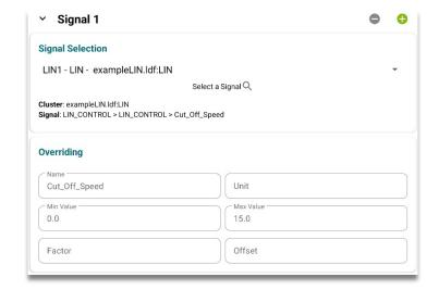
You can then open the signal search by clicking on the magnifying glass. Select a signal here and confirm with OK. If a FlexRay Channel A or B has been selected, only the signals from this channel are displayed in the signal selection dialog.
