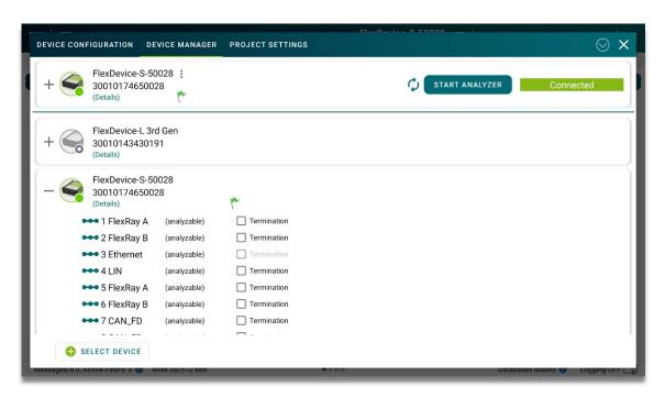
If the connection fails, please try again. If a connection cannot be established even after several attempts, please check whether the correct hardware is connected and whether the hardware is supplied with power. If the connection still cannot be established, restart the FL3X Device via the web interface or briefly disconnect the power supply to the FL3X Device.
