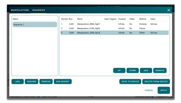
Manipulations can only be generated for a RBS bus, which was created by FL3X Config. If you create a manipulation which affects a Signal/Frame/... which isn't send by the configured RBS, the manipulation won't have any effect. Further restrictions are described in 5.4.6.
