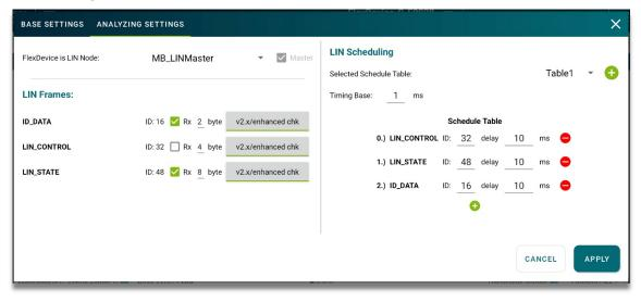
All frames from the database are listed in the configuration dialog. For each frame the ID, Rx/Tx flag, payload length and protocol version/ checksum calculation are displayed. The values are initially set with the loaded database. This information is needed for the app to receive LIN messages from a FL3X Device.
