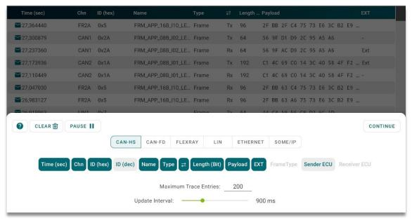
Furthermore there are app specific settings to adjust the trace behaviour. A maximum amount of trace entries can be set which is limited to 100.000 entries. Also the update interval of the trace can be changed between 400 ms and 2 seconds.
