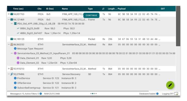
To show all information for a trace entry a database is required. If there is no database assigned to the corresponding channel or the message is not found in the database some trace column will be empty or some messages can't be expanded. A database is also required to show SOME/IP Elements instead of the raw ethernet frames.
