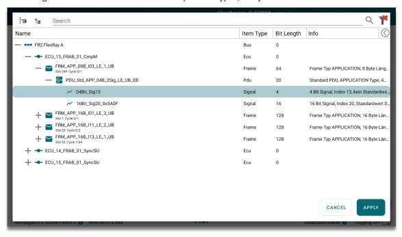
If a signal has been selected, the fields for the signal name, unit, min and max are automatically filled based on the database. These values are only valid for the current widget and can be edited. The offset and factor values allow you to subsequently adjust the received signal for each widget individually. If the fields for offset and factor are empty, the signal will not be changed.
